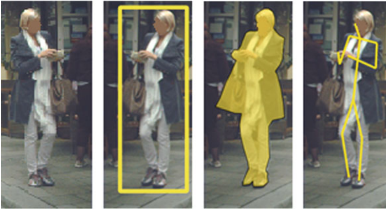
Fig. 13 Bounding box representation, shape representation, and skeleton representation
